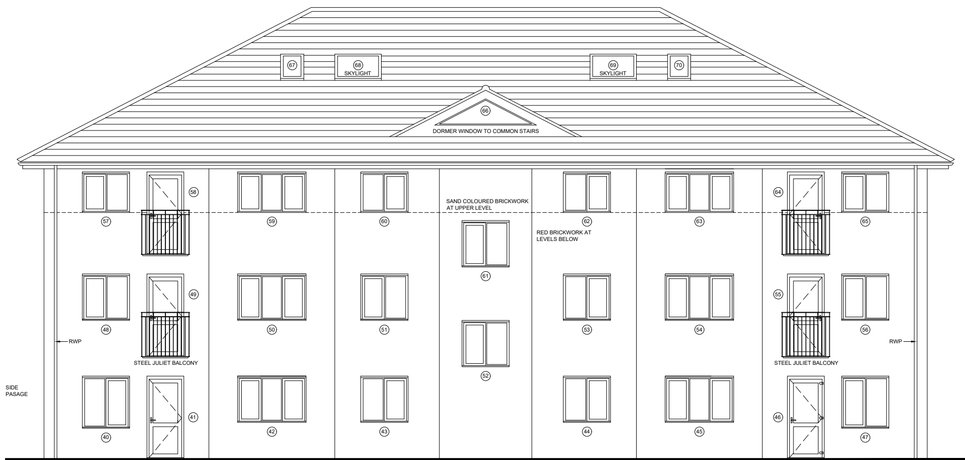
REAR ELEVATION WALLS THROUGHOUT IN FAIR FACED BRICKWORK ROOF FINISH IN ROMAN INTERLOCKING CONCRETE TILES
