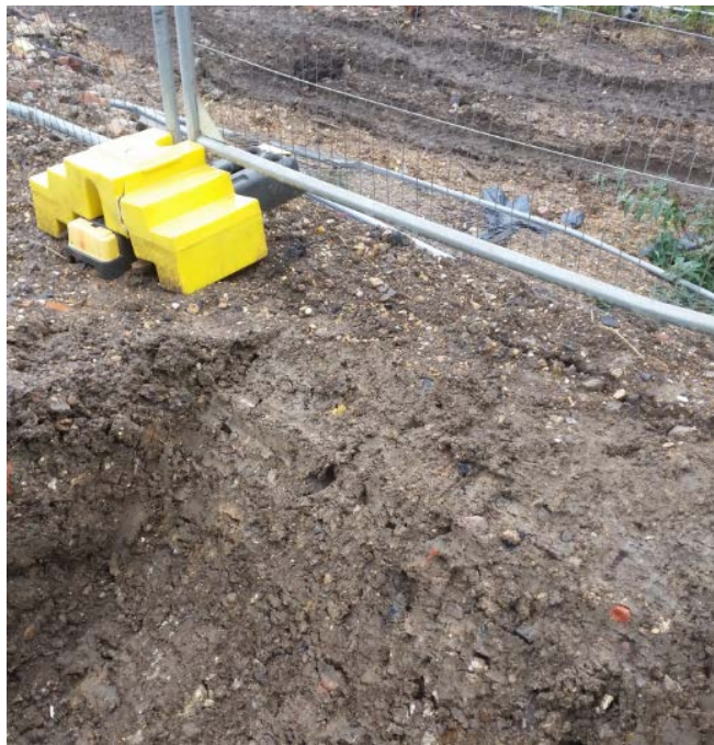
Photo 8. TP7 North bank base layer sourced from FCA Made Ground
