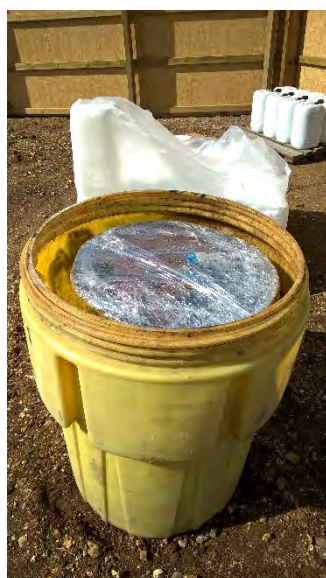
Photo 4. Damaged drums wrapped in shrink wrap and placed into plastic over drums for transport.
