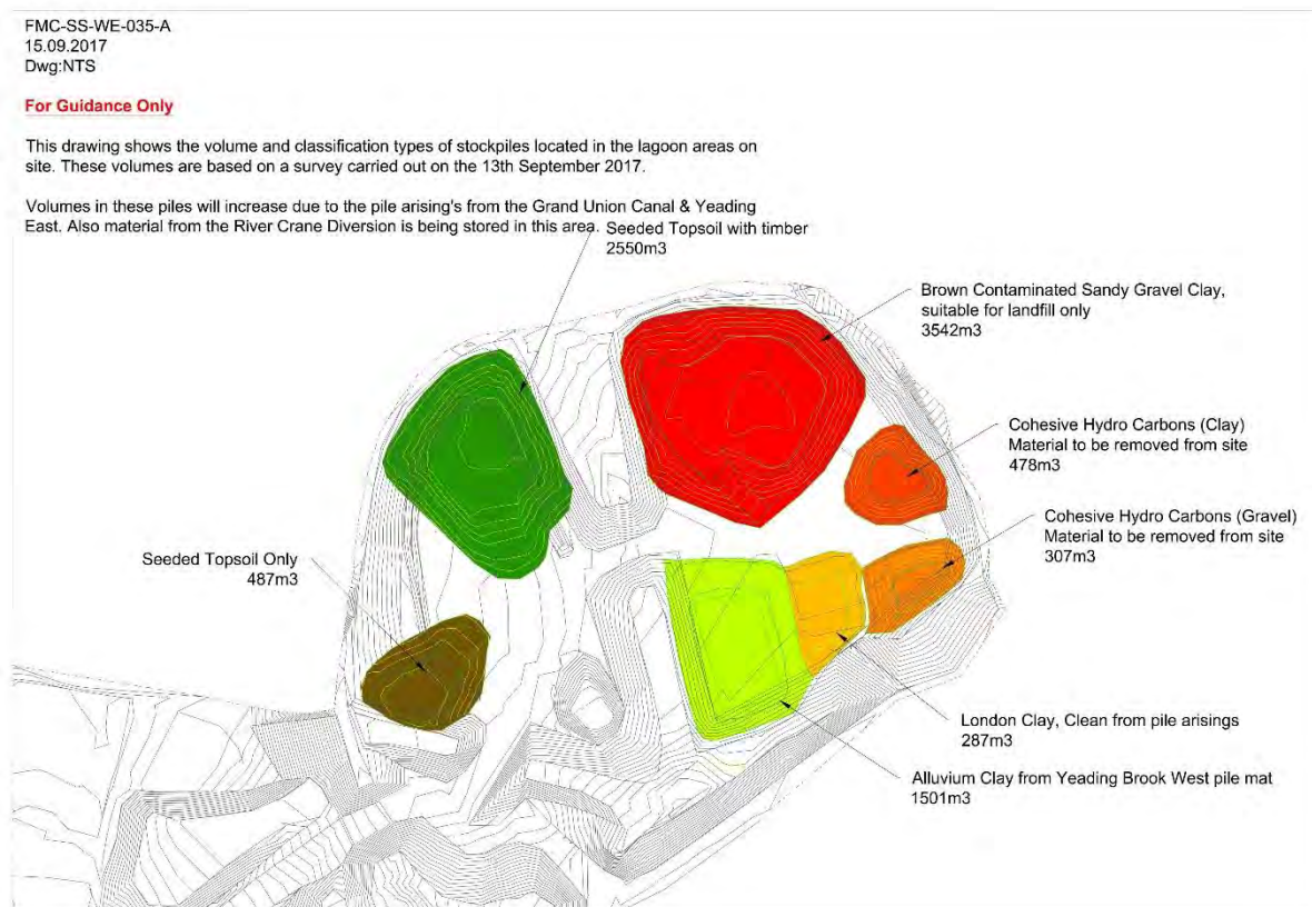
Drawing showing the location of stockpiles as of 13 th September 2017
