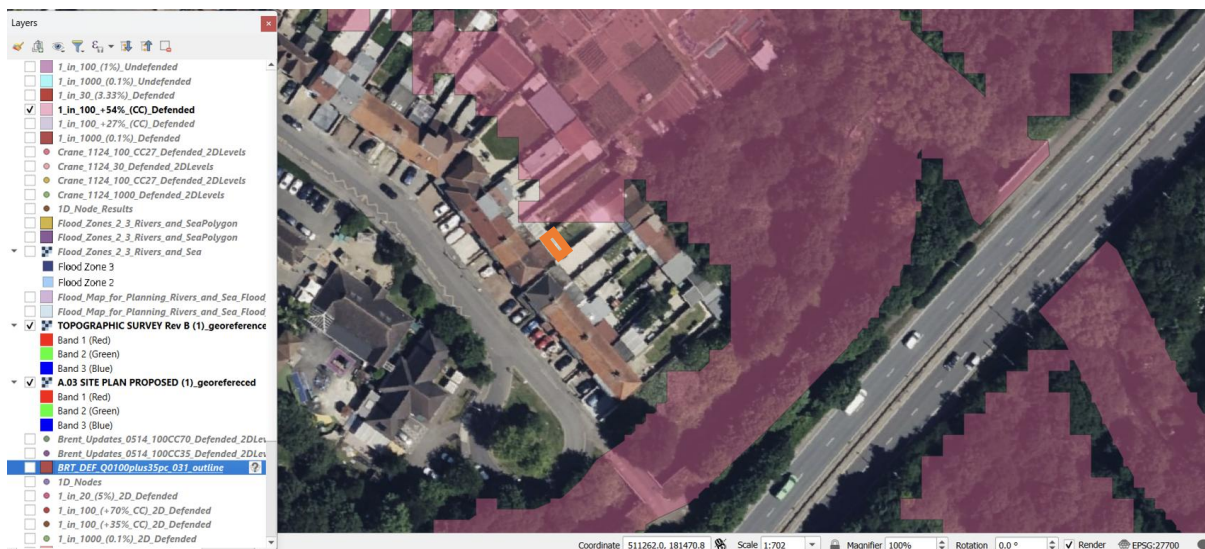
Figure 5 – 1 in 100 year plus 54% climate change defended flood extent, extension highlighted (in orange)
