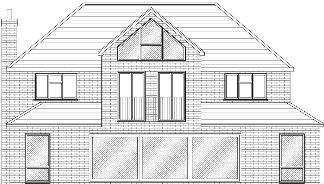
Proposed Rear Elevation Scale 1:100
