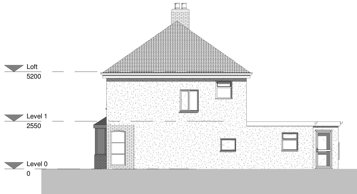
1 East elevation - Existing 1 : 100
