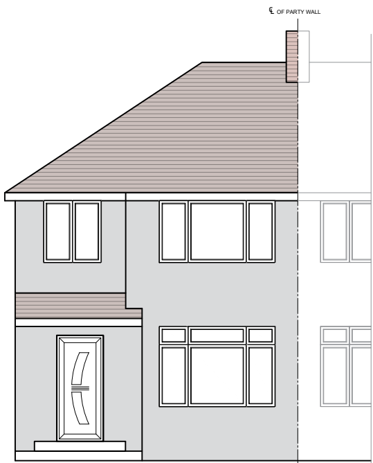
FRONT ELEVATION (existing) Scale 1:100
