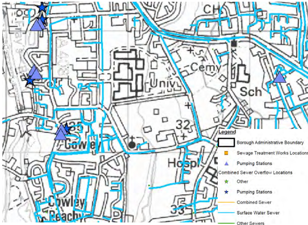
Figure 4.1 – Thames Water surface water sewer (Source: London Borough of Hillingdon Surface Water Management Plan, Appendix D, January 2013)
