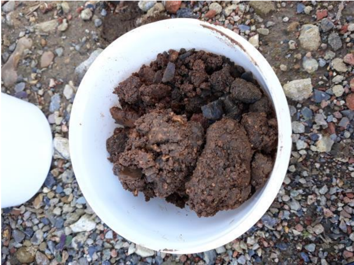
PLATE 1: Sample ES1 from TP201 (Amosite sheeting/board debris detected)
