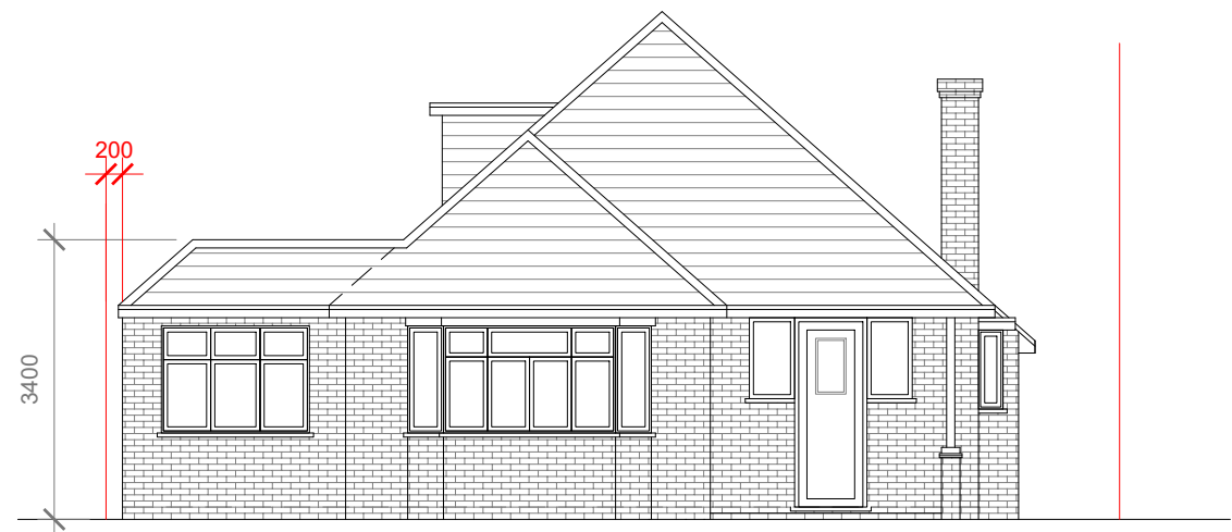
Proposed Front Elevation Scale 1:100
