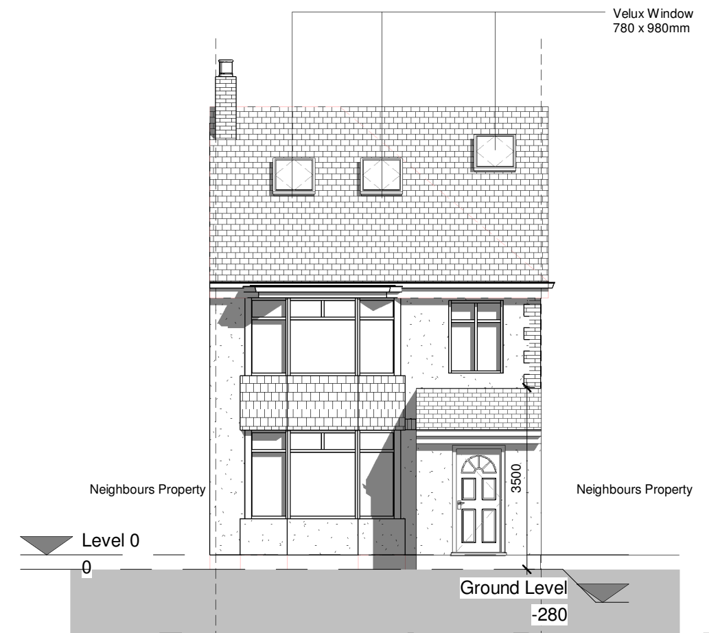
2 Front elevation - Proposed 1 : 100
