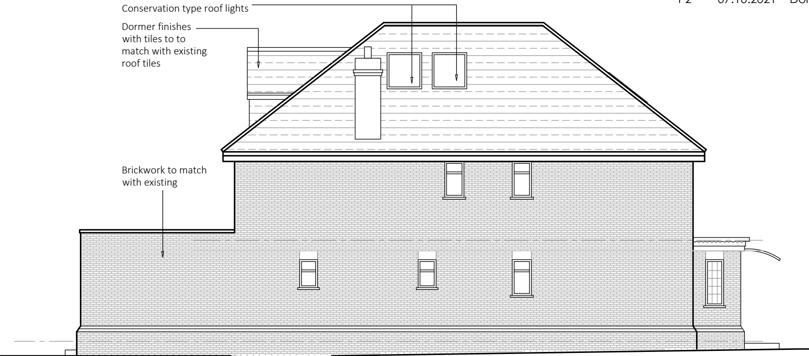
SIDE ELEVATION FACING No 38
