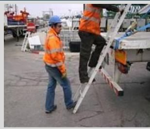
Next access trailer by means of a footed ladder, maintaining 3 points of contact – use the straps as a hand hold for the last step.
