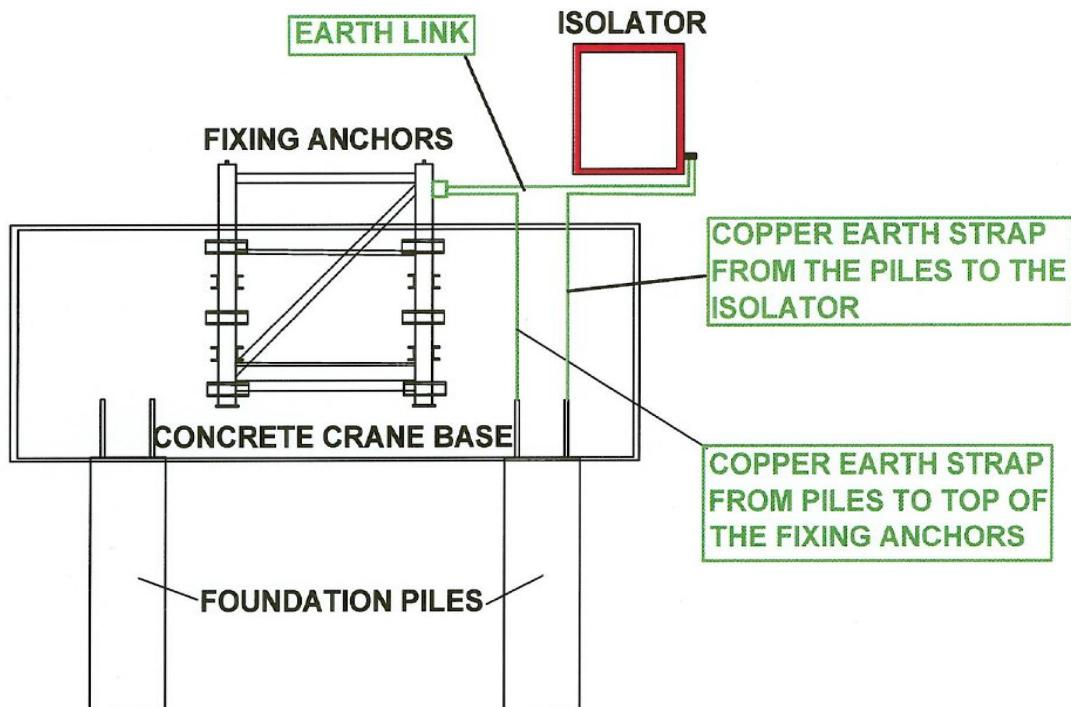
**Earthing and lightning protection is the responsibility of the client and must be in place prior to the installation of the tower crane.**
