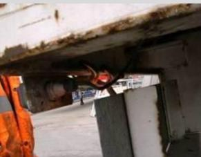
Attach hooks from the straps to a suitable Anchor point position at the front of the trailer.
