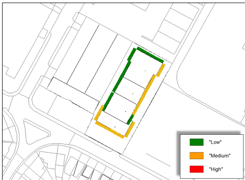
Figure 7.12: Initial AVOG Risk Assessment for Open Windows: Daytime 2 nd Floor
