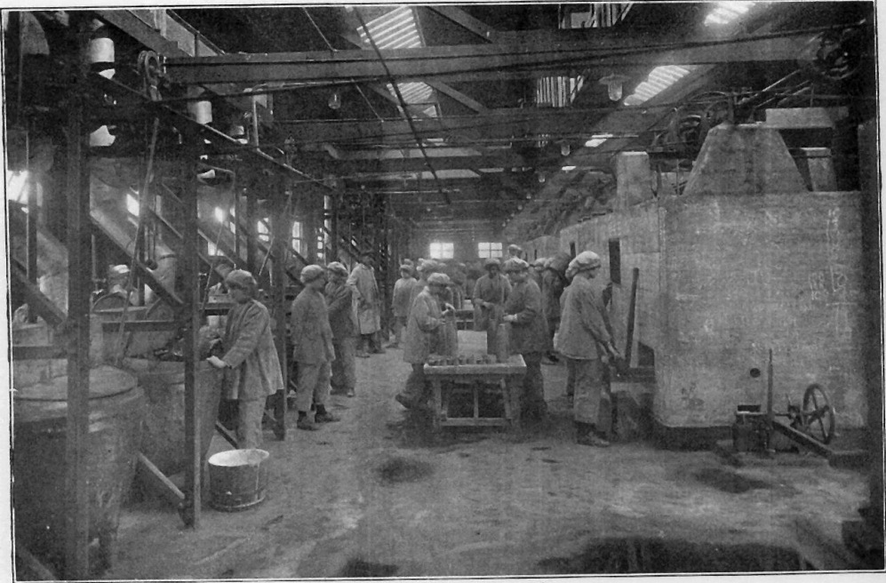
Mechanical Shell Filling, Amatol Section. Shells are filled by extruder machines inside the armoured concrete chambers on the right, so that in the event of an explosion no one would be injured.
