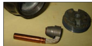
Left: baseplate and detonator removed
