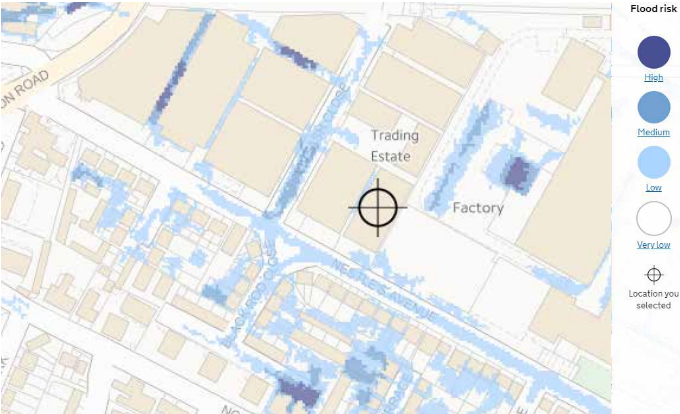
Figure 2 – Flood risk from Surface Water
