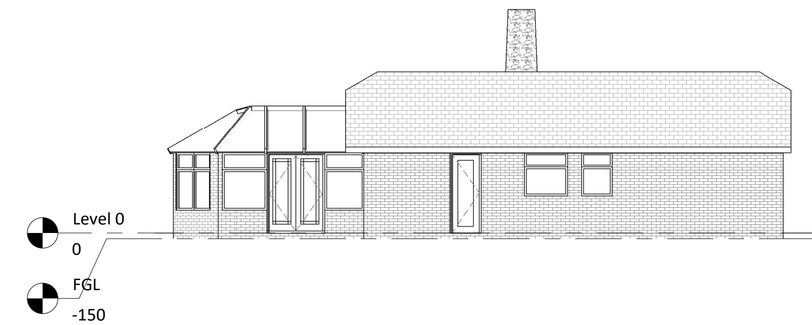
Existing Right Side Elevation 1 : 100
