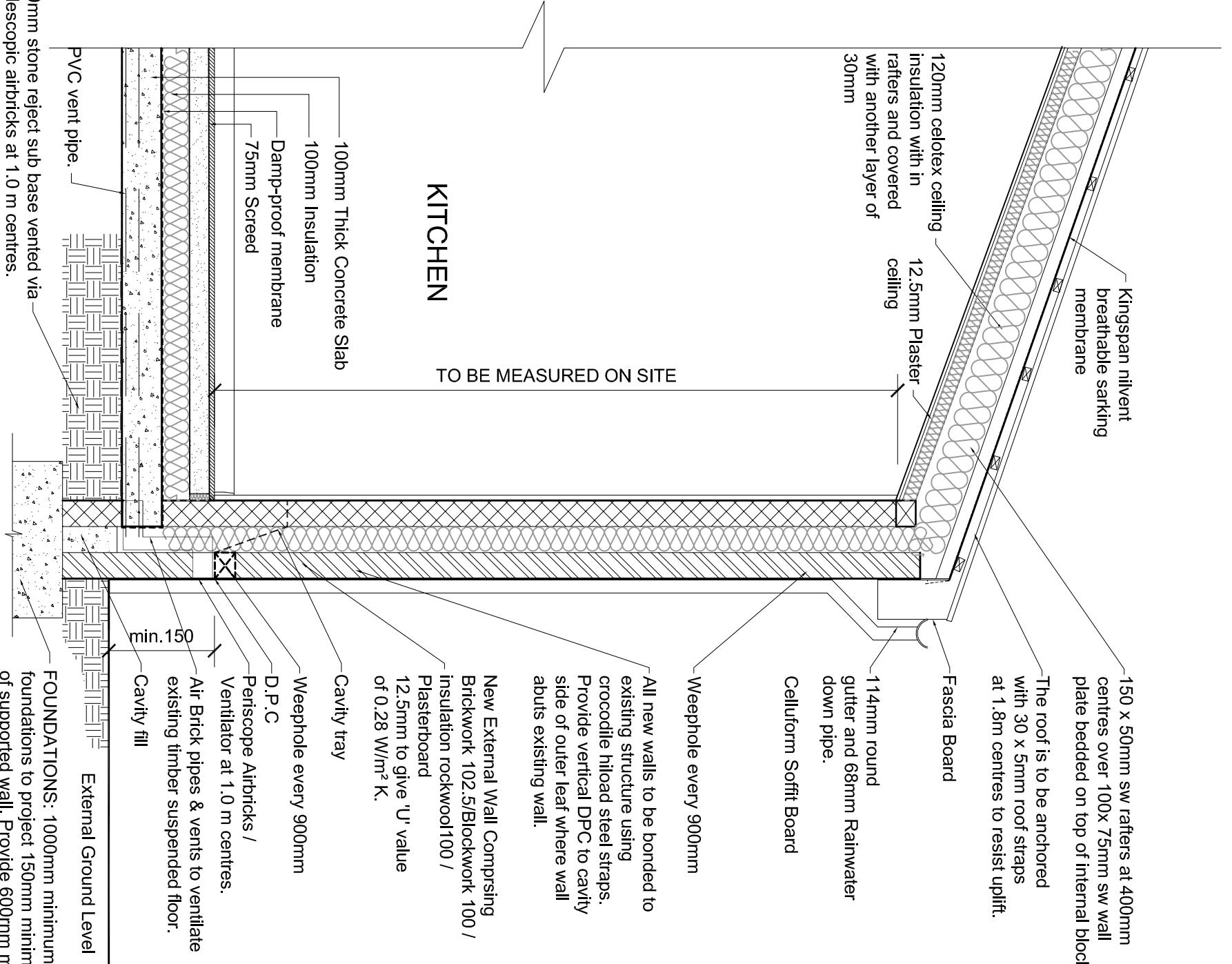
40mm stone reject sub base vented via telescopic airbricks at 1.0 m centres. Polythene membrane laid directly on top of sub base. Layer of sand blinding laid over this membrane.
