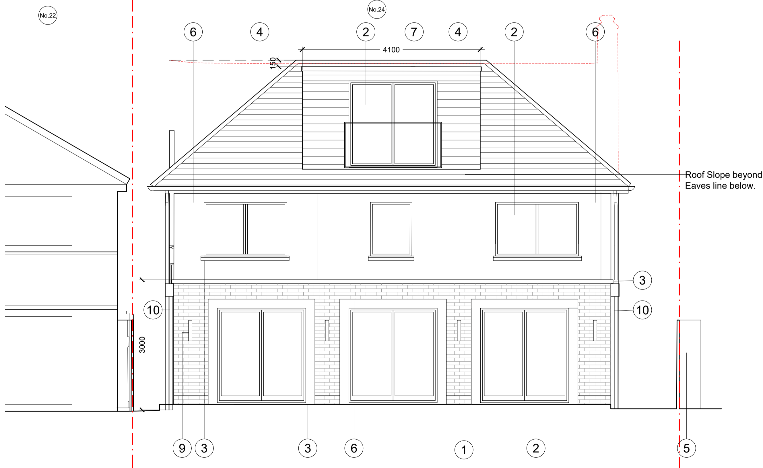
2 PROPOSED REAR ELEVATION 1:50 @ A1, 1:100 @ A3
