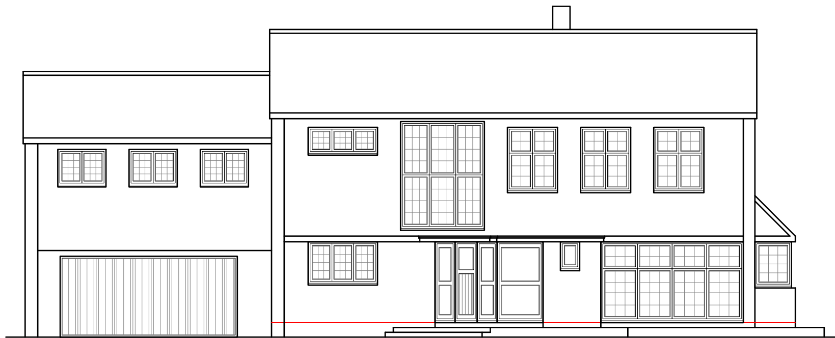
EXISTING FRONT ELEVATION 1:100
