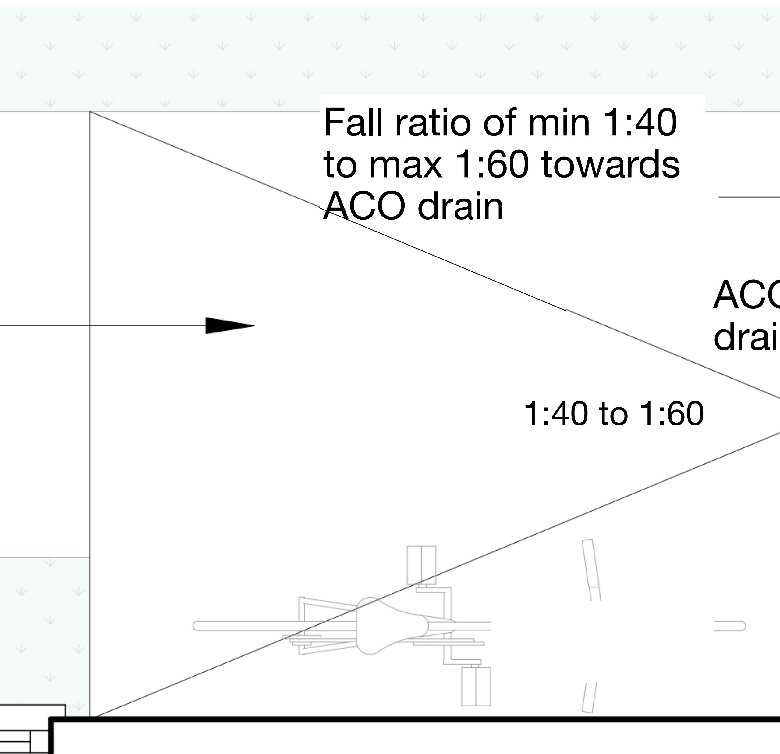
Fall ratio of min 1:40 to max 1:60 towards ACO drain
