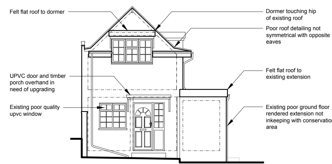
Front Elevation As Existing 1:100
