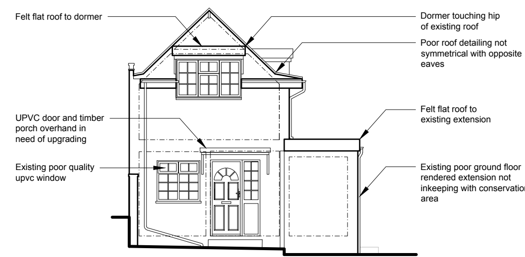
Front Elevation As Existing 1:100
