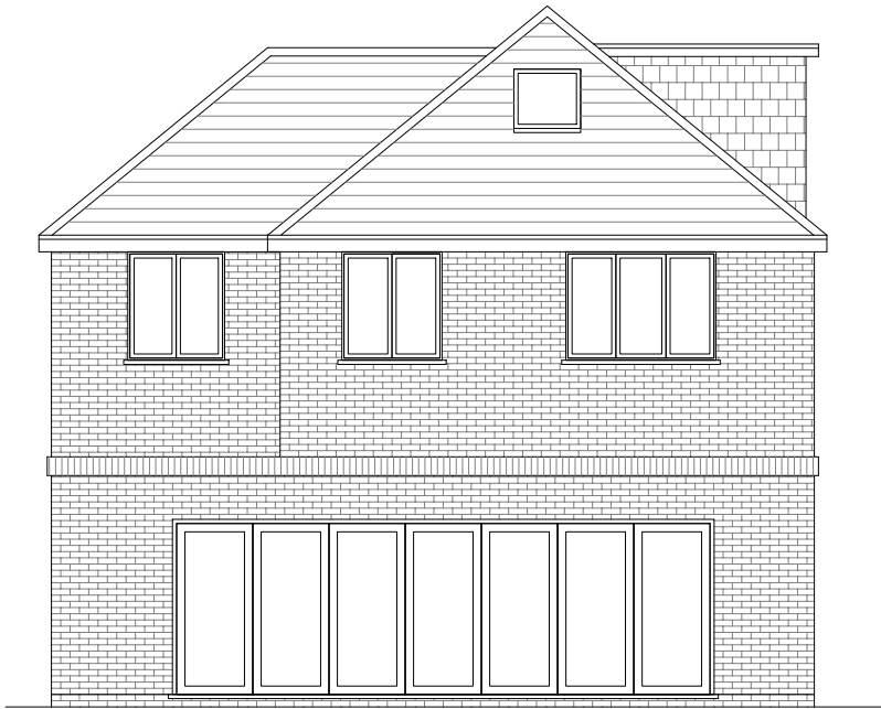
Existing Rear Elevation Scale 1:100
