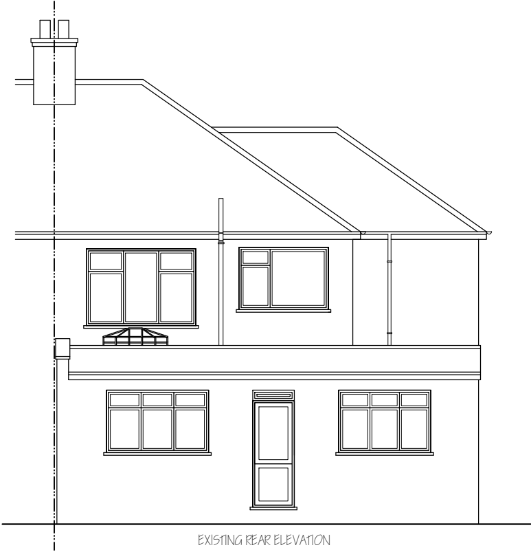
EXISTING REAR ELEVATION
