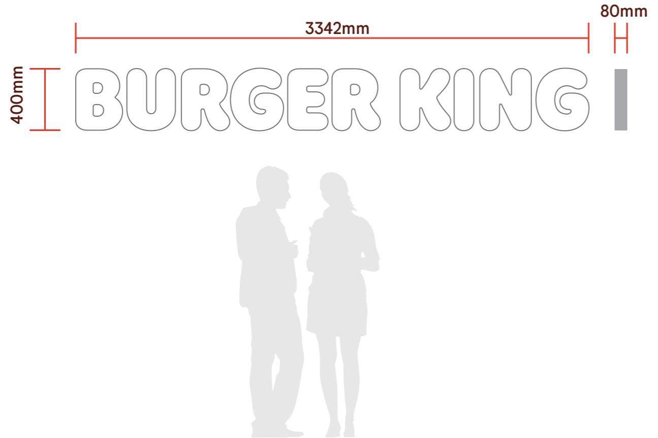
Internally illuminated letterset, constructed from aluminium.
