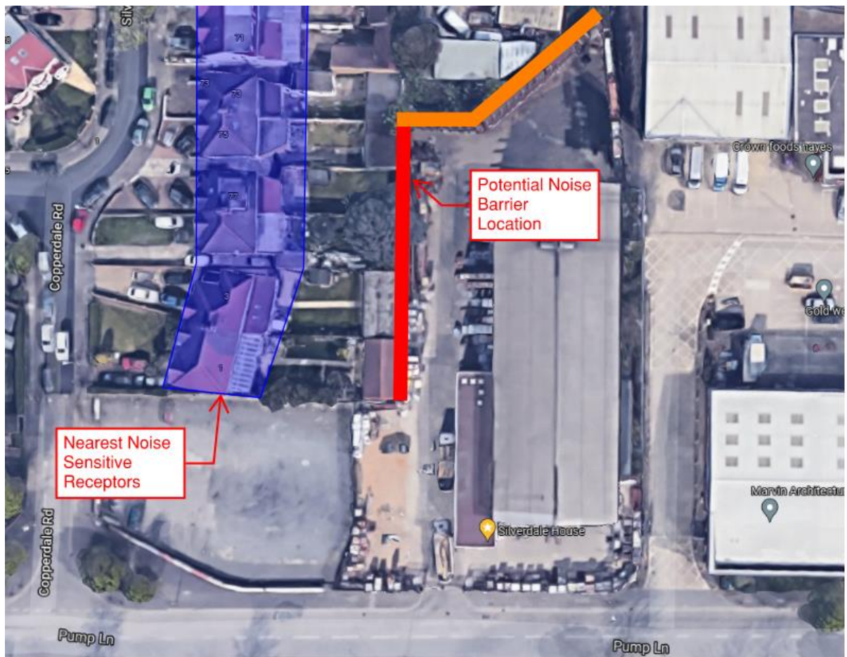
Figure 3 - Potential Noise Barrier Location
