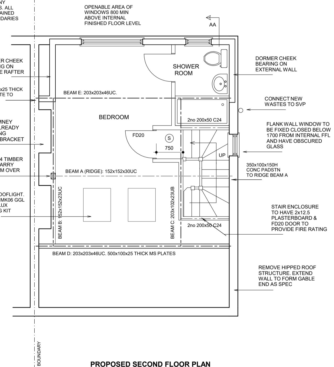
(S) SELF CONTAINED MAINS OPERATED INTERLINKED OPTICAL SMOKE ALARM SYSTEM IN ACCORDANCE WITH BS5839 OR BS5446. ALARMS TO HAVE BATTERY BACK UP. DETECTORS 300mm FROM WALLS
