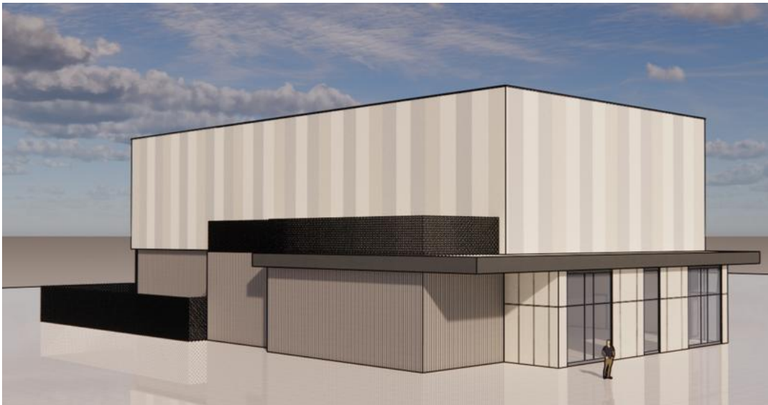
Sketch of the massing concept of the proposed Data Centre, note the admin / entrance is stepped down and canopy wraps around
