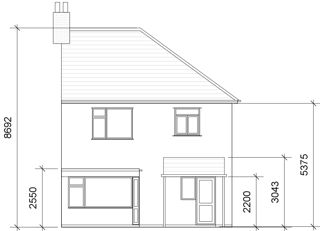
Existing Rear Elevation
