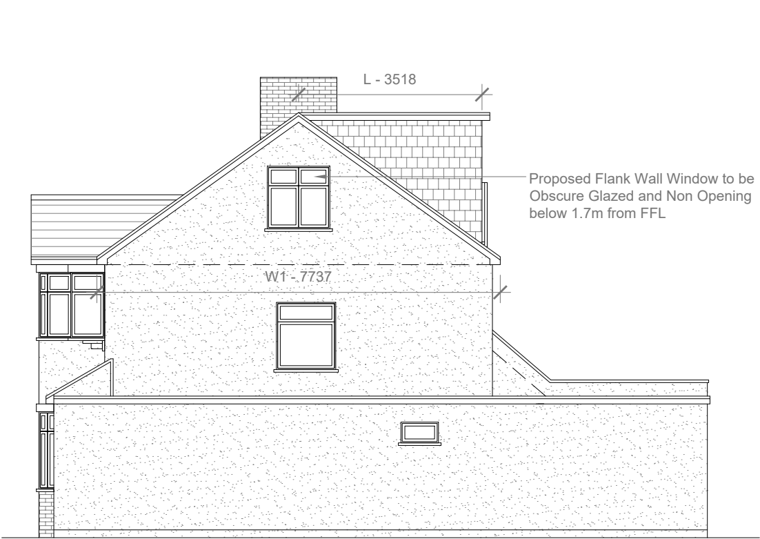
Proposed Side Elevation Scale 1:100
