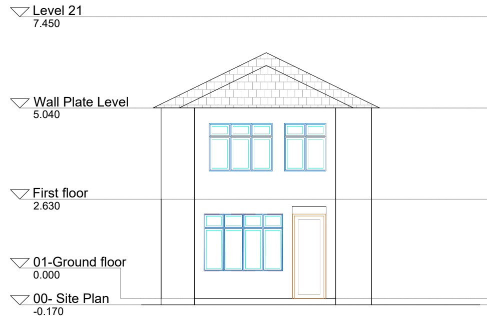
7 South elevation - Existing 200 SCALE 1 : 100
