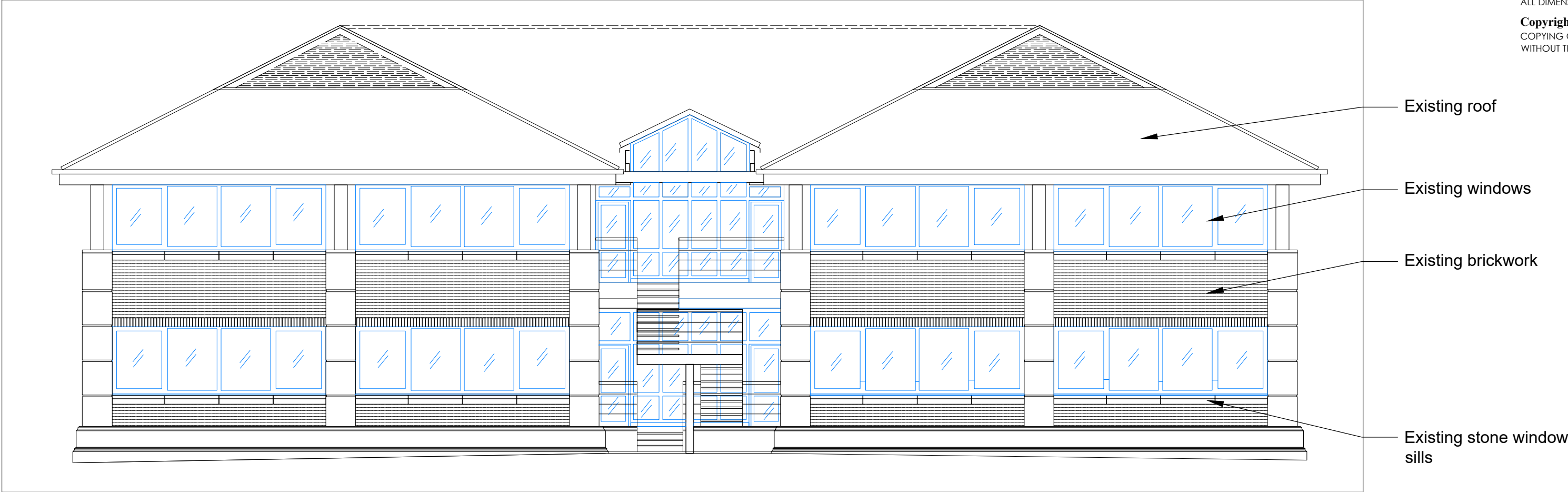
EXISTING WEST ELEVATION
