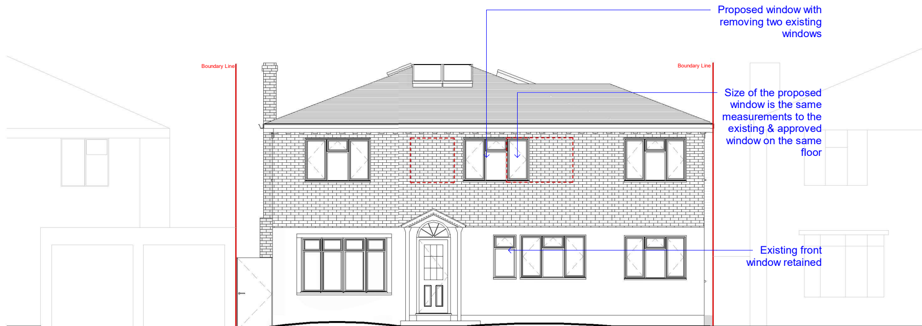
Front elevation- Existing 1 : 100
