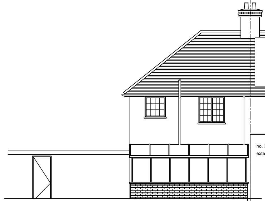
REAR ELEVATION AS EXISTING
