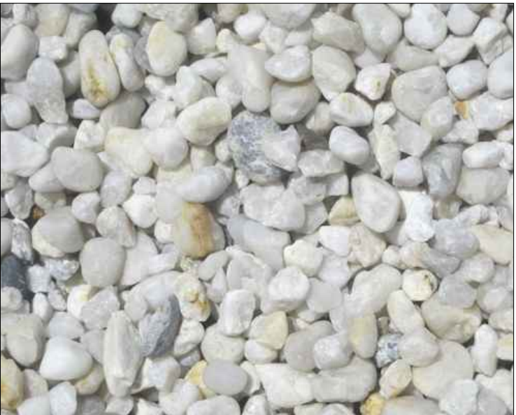
White quartz gravel strip to building edge
