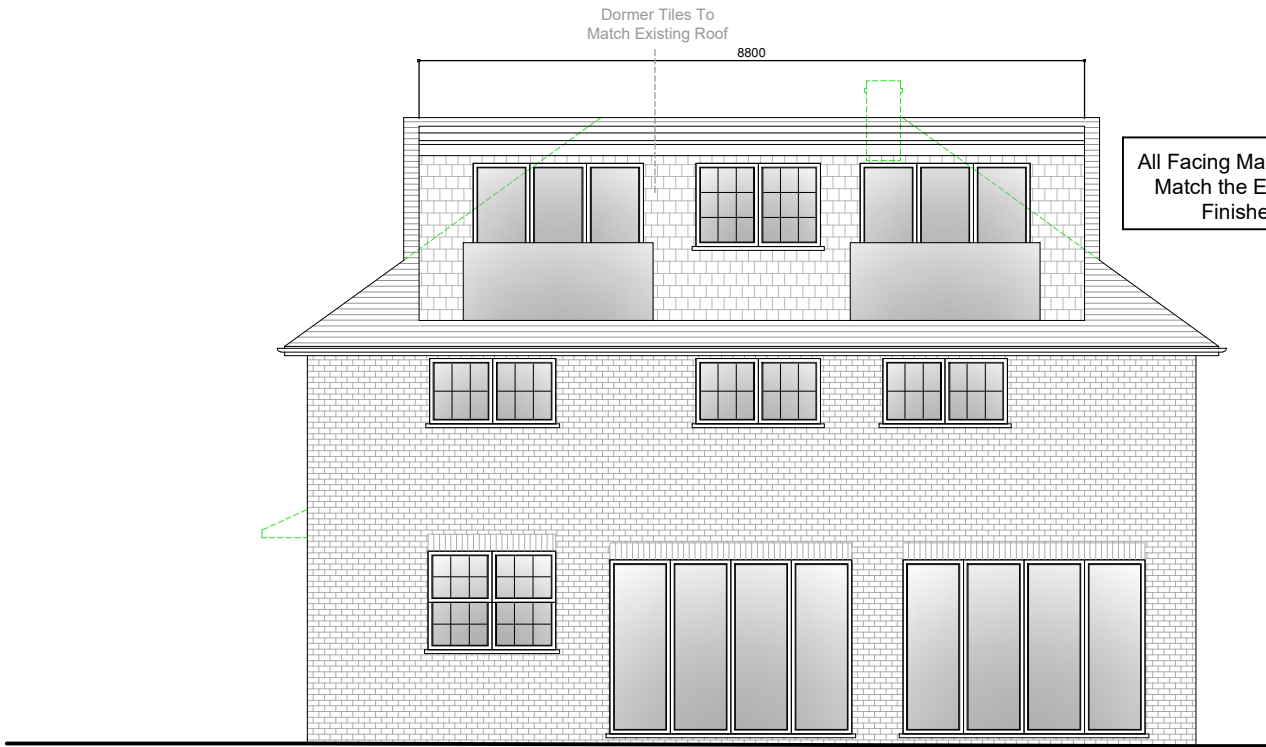
Proposed Rear Elevation Scale 1:100
