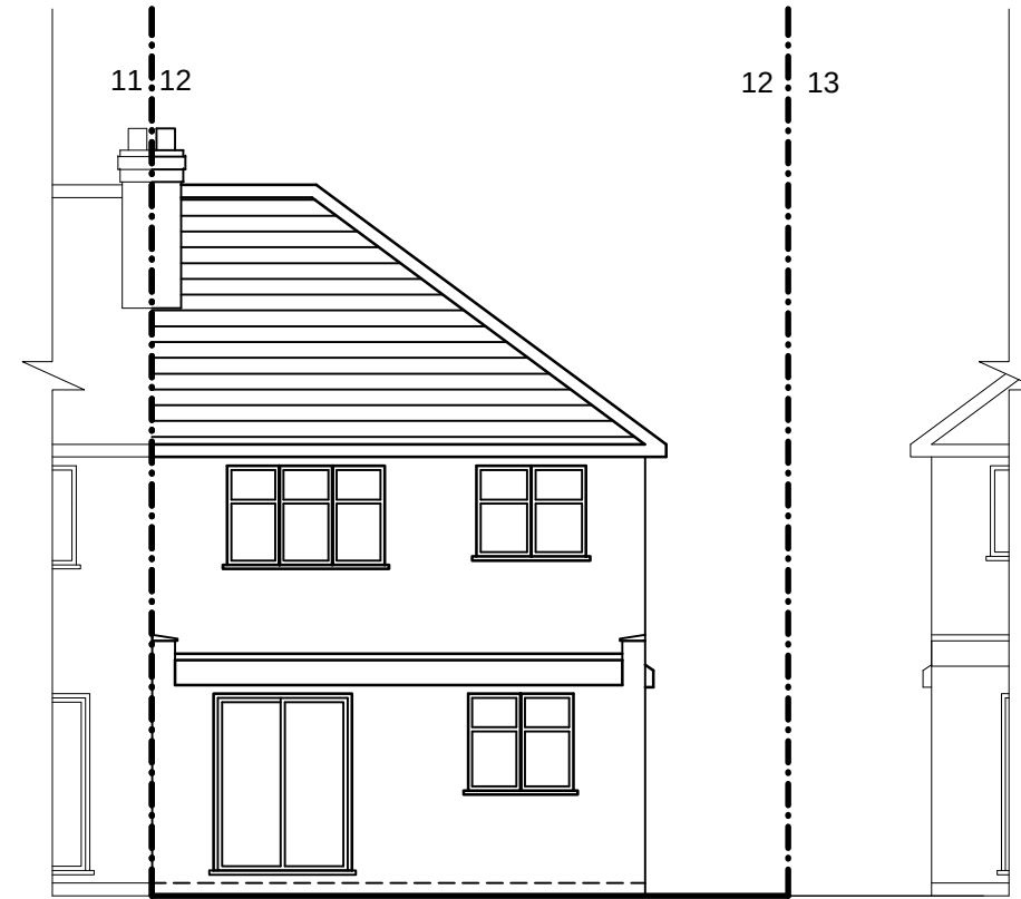
REAR ELEVATION EXISTING (BOUNDARY WALL/FENCE & SHED ARE OMITTED FOR CLARITY OF ELEVATION)
