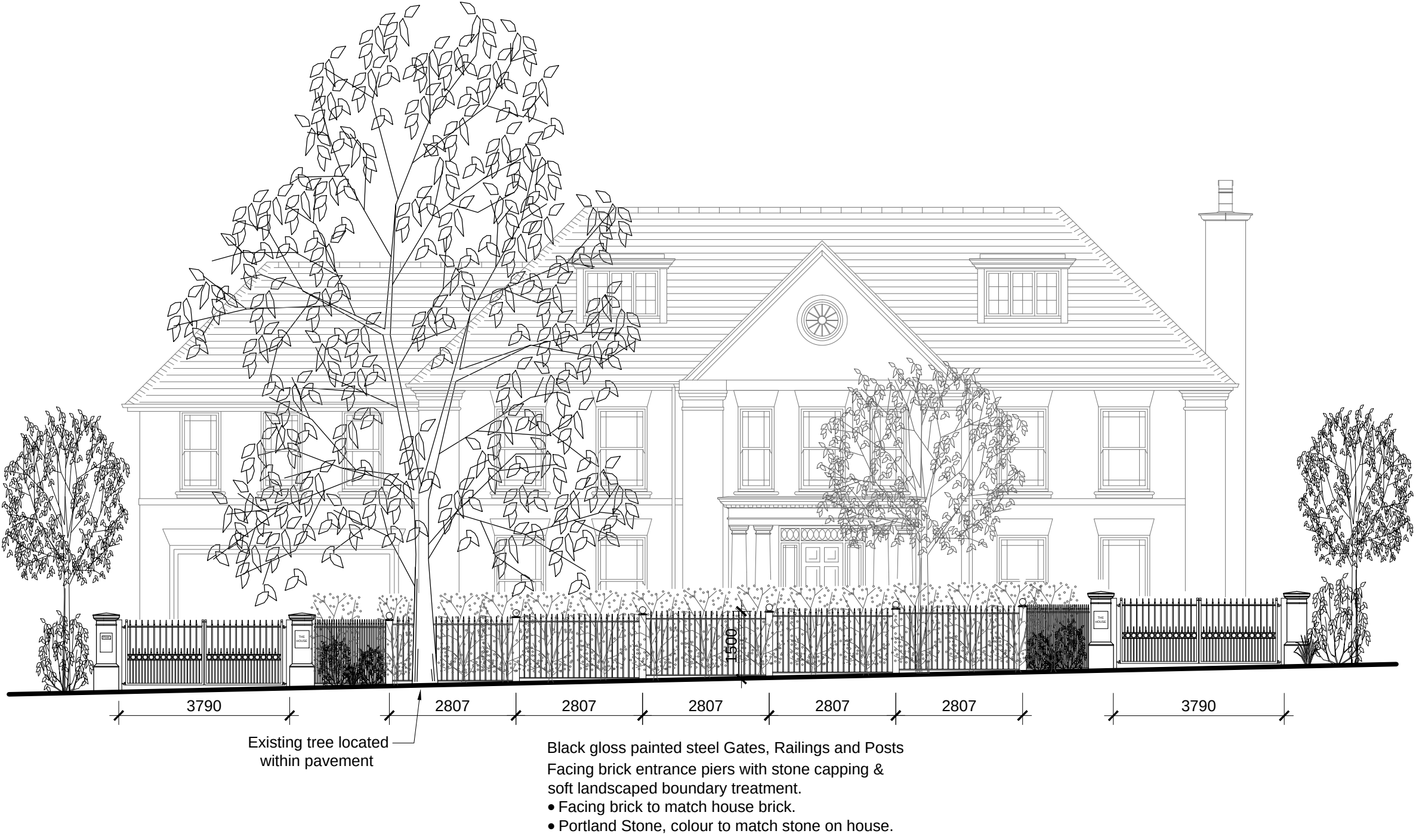
Entrance Gate and Railings Elevation, 1:100
