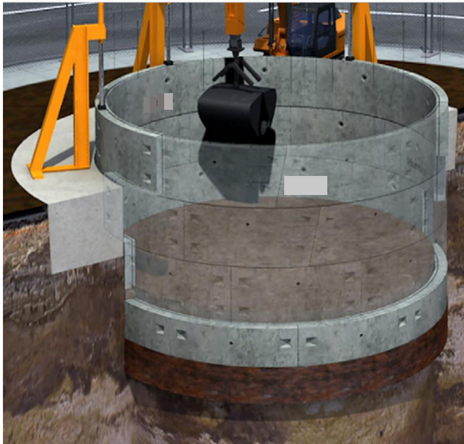
Fig. Visual representation of shaft construction using Jack-down technique
