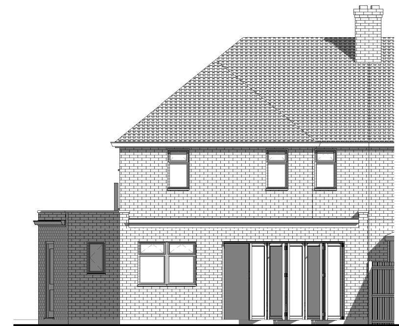
3 Existing Rear Elevation. 1 : 100
