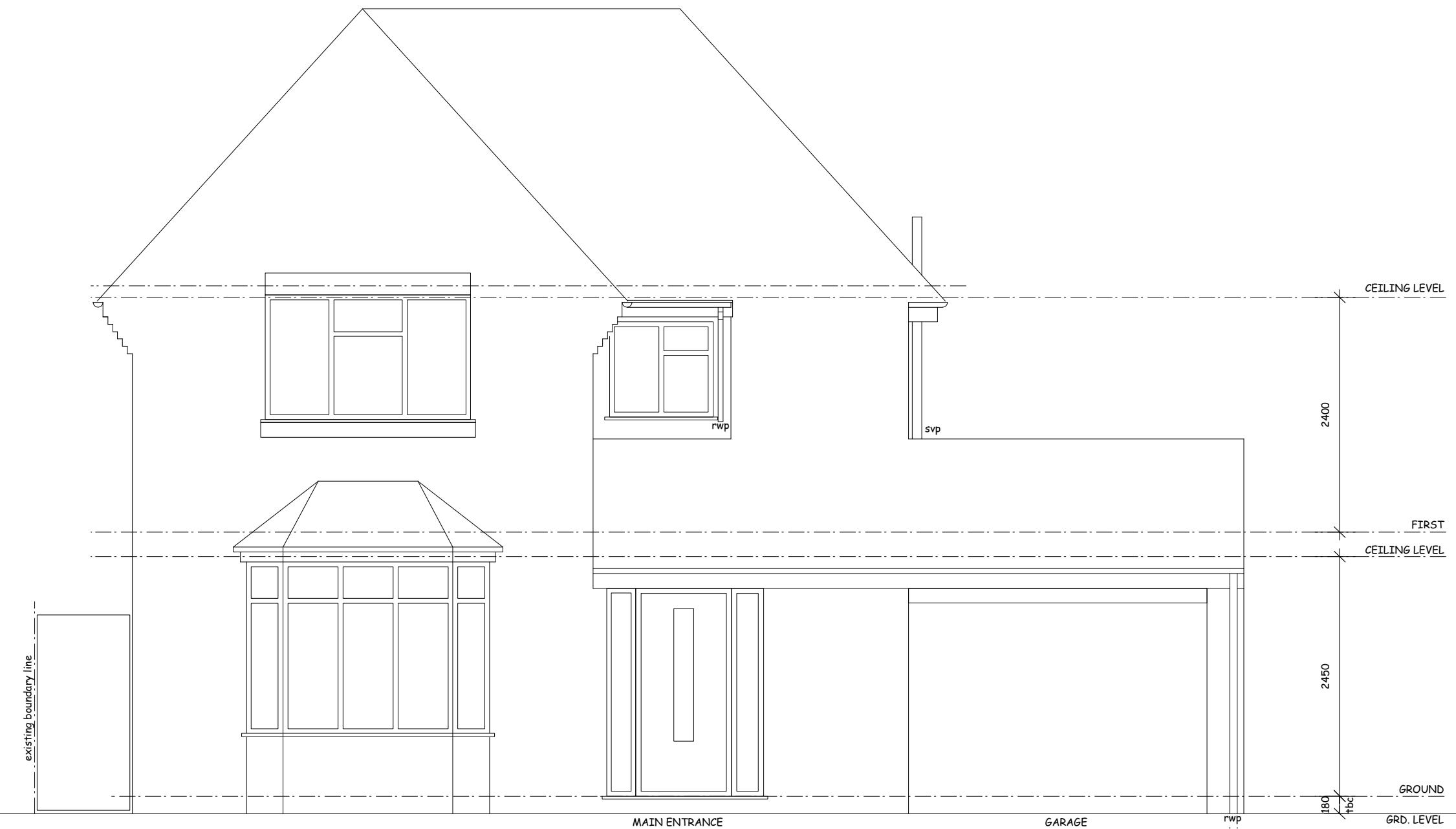
43 OD E04p1 EXISTING ELEVATION 1 0 1m 2m 3m 4m 5m
