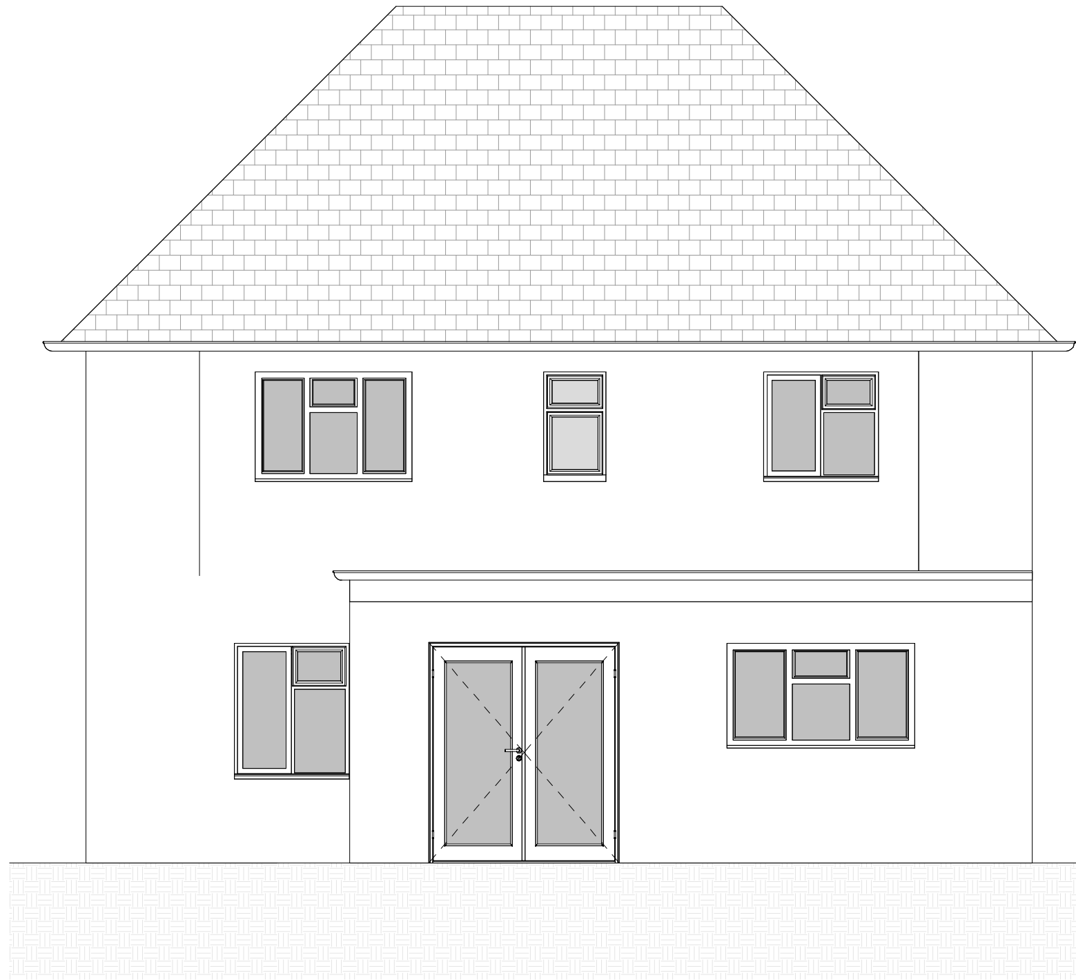
2 EXISTING REAR ELEVATION 1 : 50
