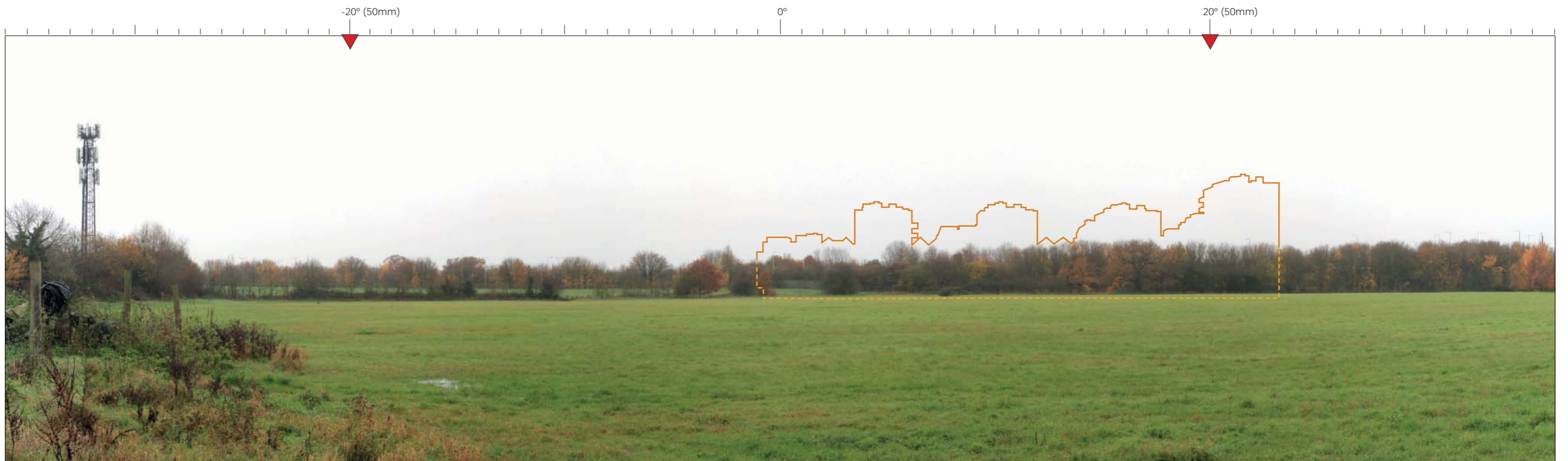
23.1.2. Wireline of proposed units at a viewing distance, this is the distance from eye to paper to gain a true representation of the image. VD at 30cm
