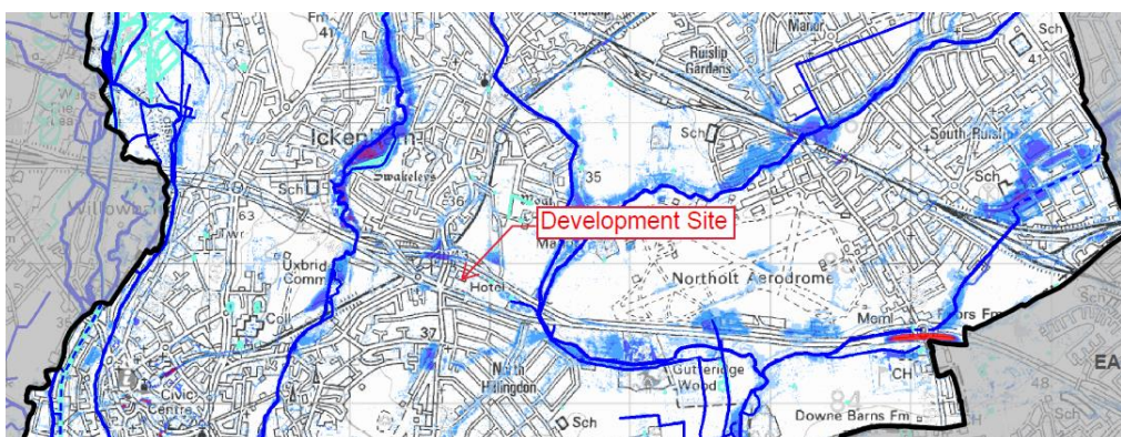
Extract from LBH PFRA Figure B-3.1 – Surface Water Depth – 1 in 100 plus climate change chance of rainfall event occurring in any given year.
