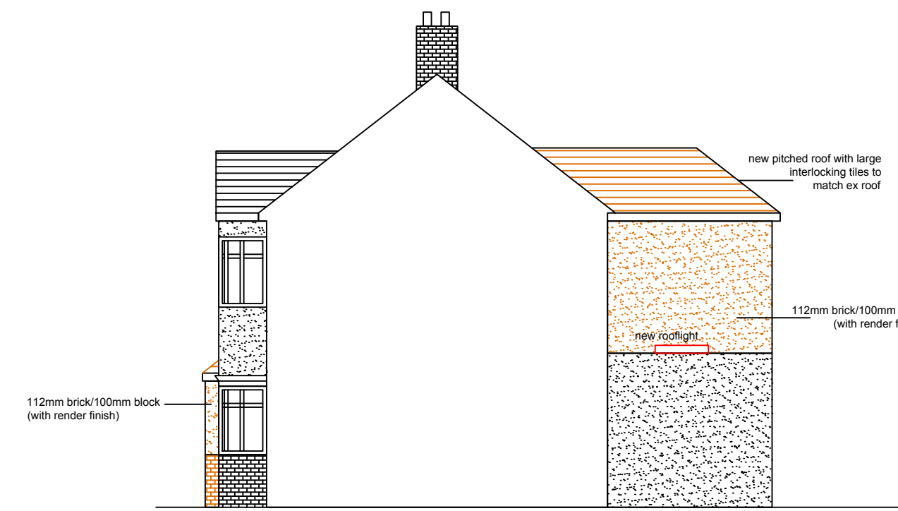
proposed side elevation from no 55 1:100
