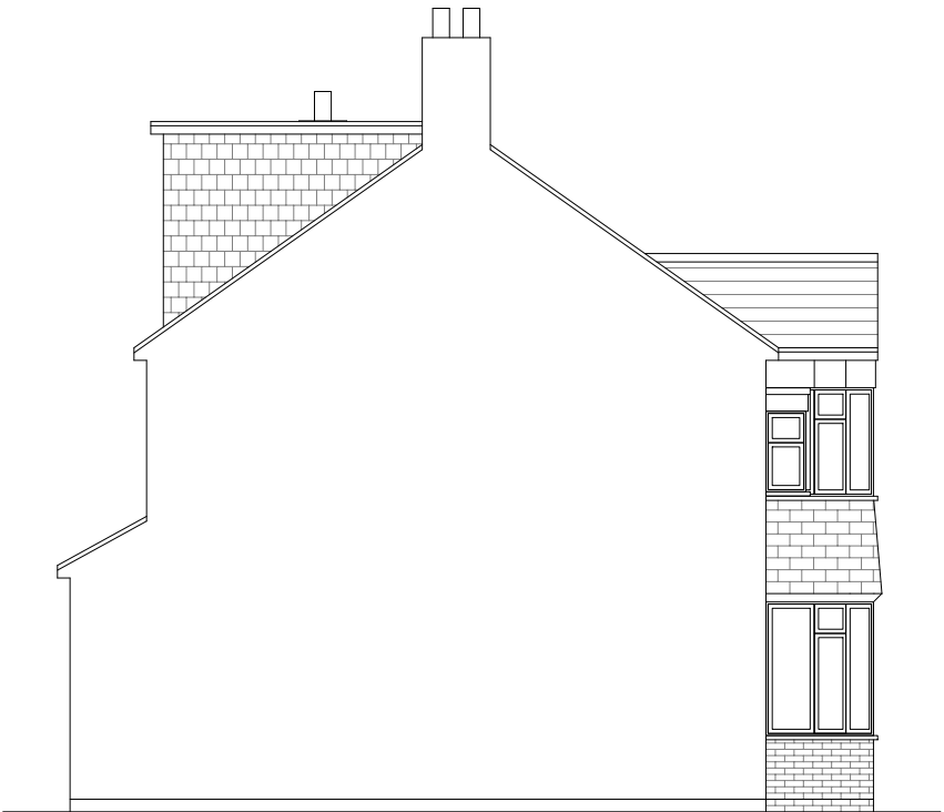
Proposed Side Elevation Scale 1:100
