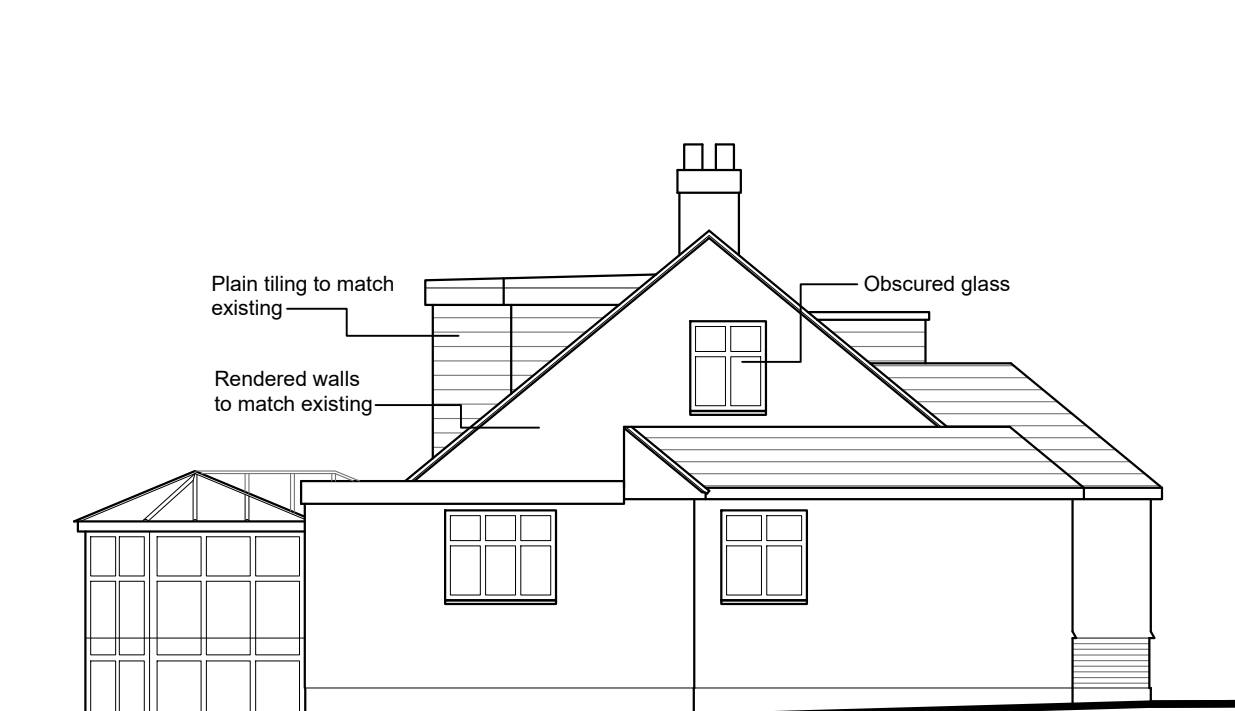
PROPOSED SIDE (EAST) ELEVATION
