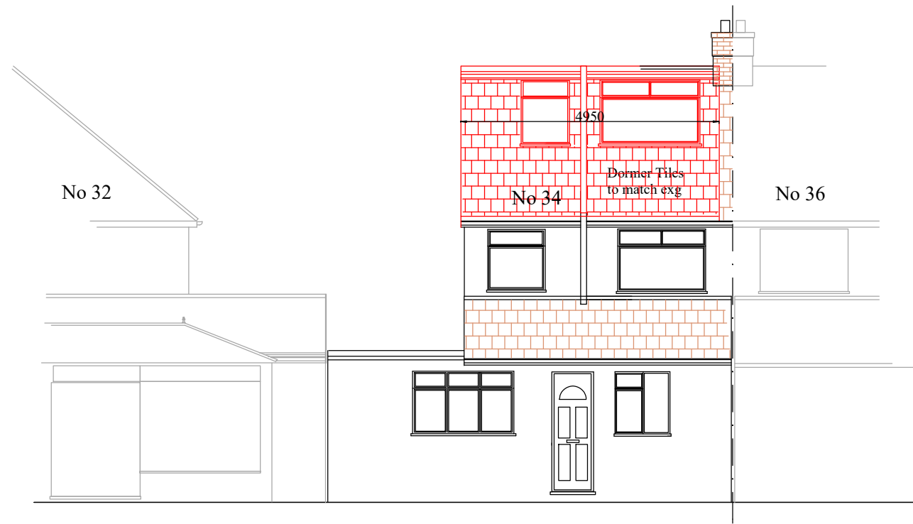
PROPOSED REAR ELEVATION
